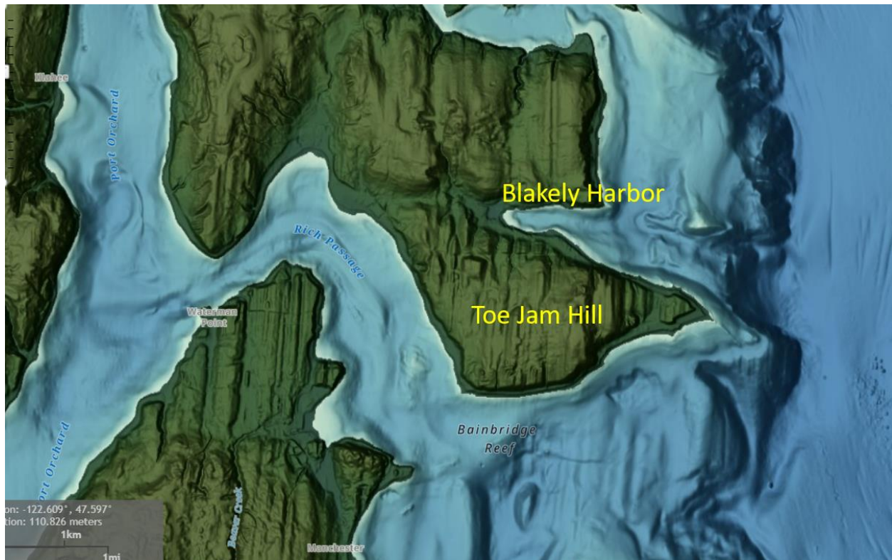
LIDAR image of the rock surface around Rich Passage. The strong north-south hills and valleys were sculpted by the retreating ice sheet as the Puget Sound lobe melted. Toe Jam Hill and the Blakely Harbor Inlet show a contrary east-west grain.
